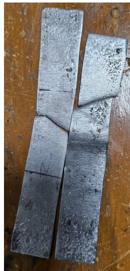
Failed mild steel specimens (under uni-axial tension)
