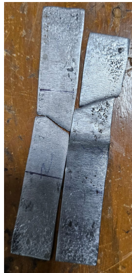
Failed mild steel specimens (under uni-axial tension) ◀ ◻ ▶
