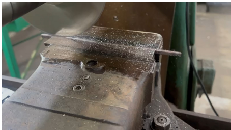
Figure 1: Milling machine used to cut grooves
