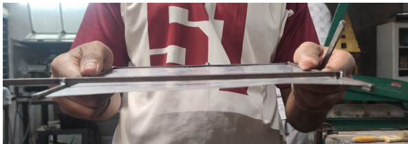
Figure 7: Imperfections in Plate
