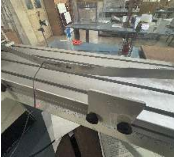
Figure 5: Buckling of 1mm specimen
