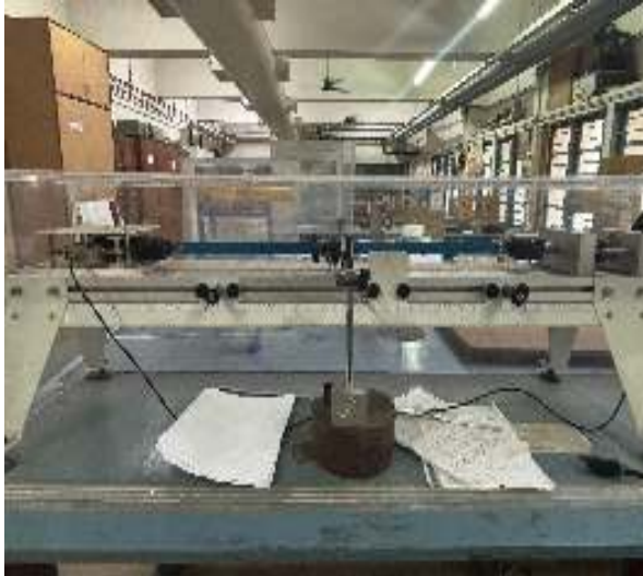
Figure 1: Dial Gauge setup
