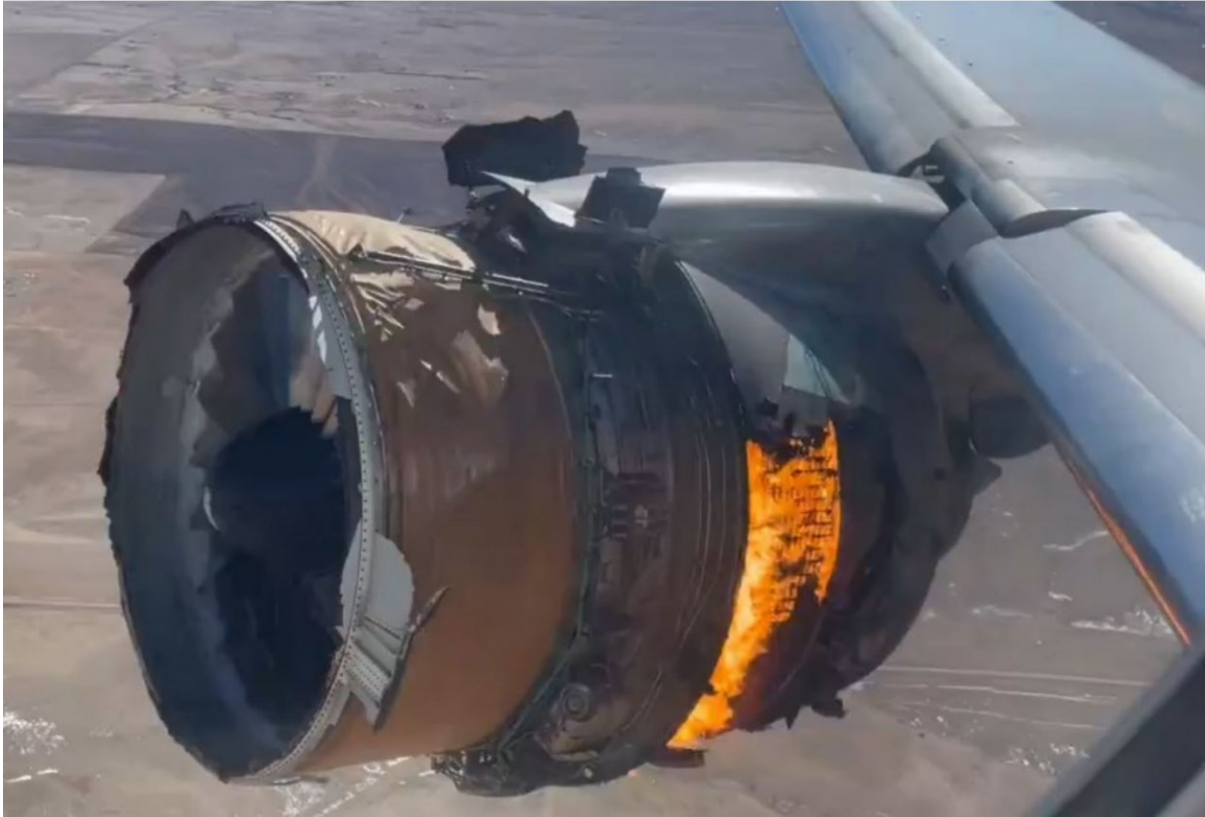
Figure 1. Still image from passenger in-flight video showing engine nacelle damage and under-cowl fire about 11 minutes after fan blade separation (Courtesy Boeing via YouTube).
