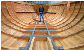
A wooden ship hull Lyman-Morse Builds New in Wood and Glue - Professional BoatBuilder Magazine 2024
