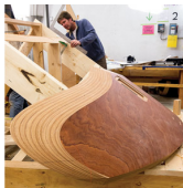
A wooden ship hull Lyman-Morse Builds New in Wood and Glue - Professional BoatBuilder Magazine 2024
