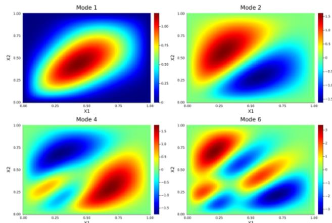
*Example: Thin plate (pinned) under shear loading*
