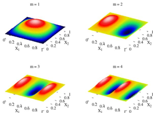
*Example: Thin plate (pinned) under axial loading*
