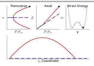
**Example**: A pinned-pinned beam undergoing axial loading.
