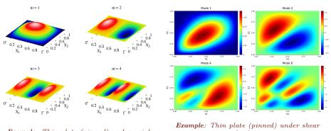
Example: Thin plate (pinned) under axial loading
