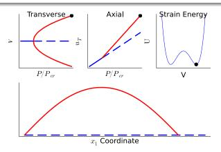
Example: A pinned-pinned beam undergoing axial loading.
