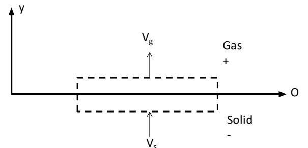
Hence for component (f) and (a):  $\rho_g Y_{ig} (\bar{v}_g + \bar{V}_{ig}) - \rho_s Y_{is} (\bar{v}_s + \bar{V}_{is}) = 0$
